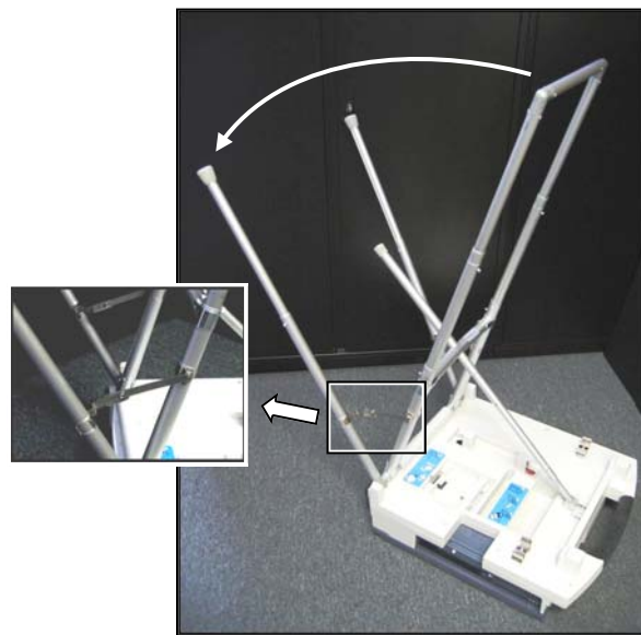
STEP FIVE — Now, pull the outside legs away from the unit. The legs and inside support bar will form a “V” shape. Further secure the machine by making sure the leg brackets are straightened.
